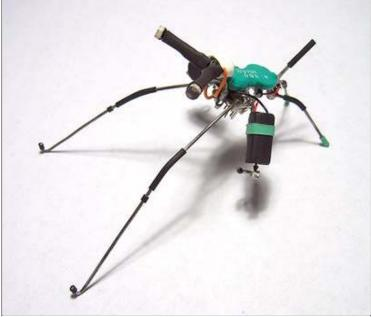
This dual-motor vibrobot has the ends of paperclips soldered to two pager motors. Each motor is connected to a <u>CdS cell</u> so the more light each "eye" gets, the more the motor on that side fires. It's great to watch it react to a flashlight.
